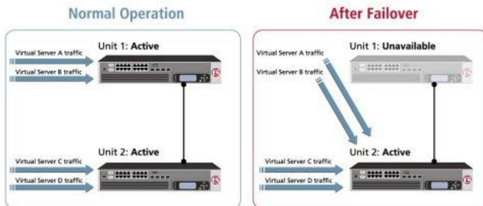
The figure shows an active-active configuration in which units 1 and 2 are both in active states. With this configuration, failover causes the following to occur:
